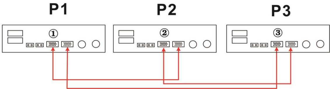
**WARNING:** Do not connect the current sharing cable between the inverters which are in different phases. Otherwise, it may damage the inverters.
