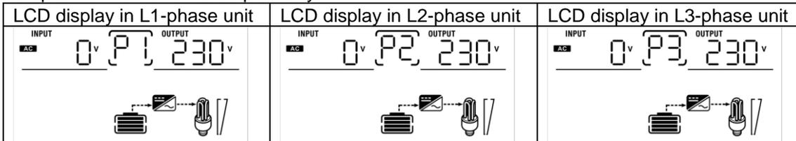
Step 4: Switch on all AC breakers of Line wires in AC input. If AC connection is detected and three phases are matched with unit setting, they will work normally. Otherwise, the AC icon will flash and they will not work in line mode.
