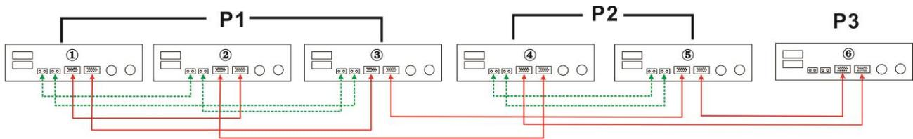
Three inverters in one phase and only one inverter for the remaining two phases:
