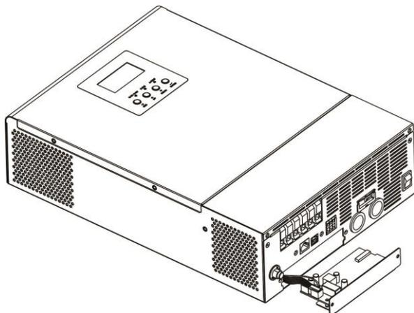
**Step 3:** Connect the cables to the parallel board, and insert the board back to the unit by fixing two screws.
