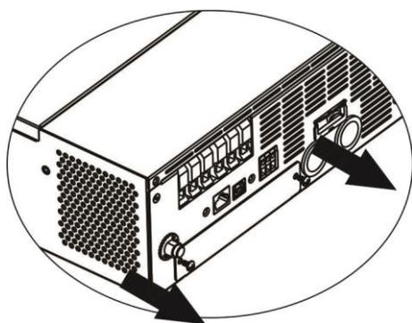
**Step 2:** Disconnect the cable and remove the dummy board.
