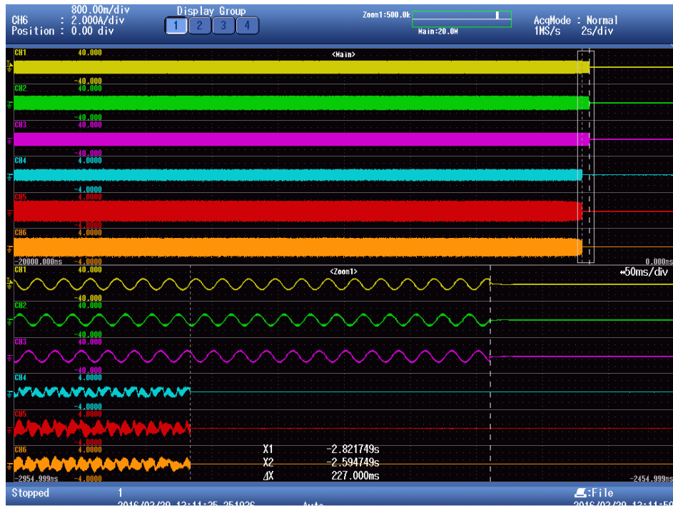
Fundamental of I_{AC} at balance condition = 53mA
