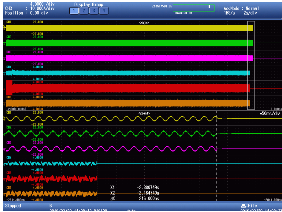
Fundamental of I_{AC} at balance condition = 33mA
