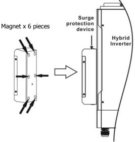
**Step 2:** Connect the OUTPUT of SPD to AC grid connectors of Hybrid Inverter. The INPUT of SPD is connected to AC utility.
