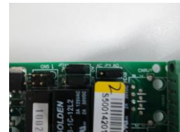
Fig. 5 AO and AC silk printings indicates each 3-pin connector status
